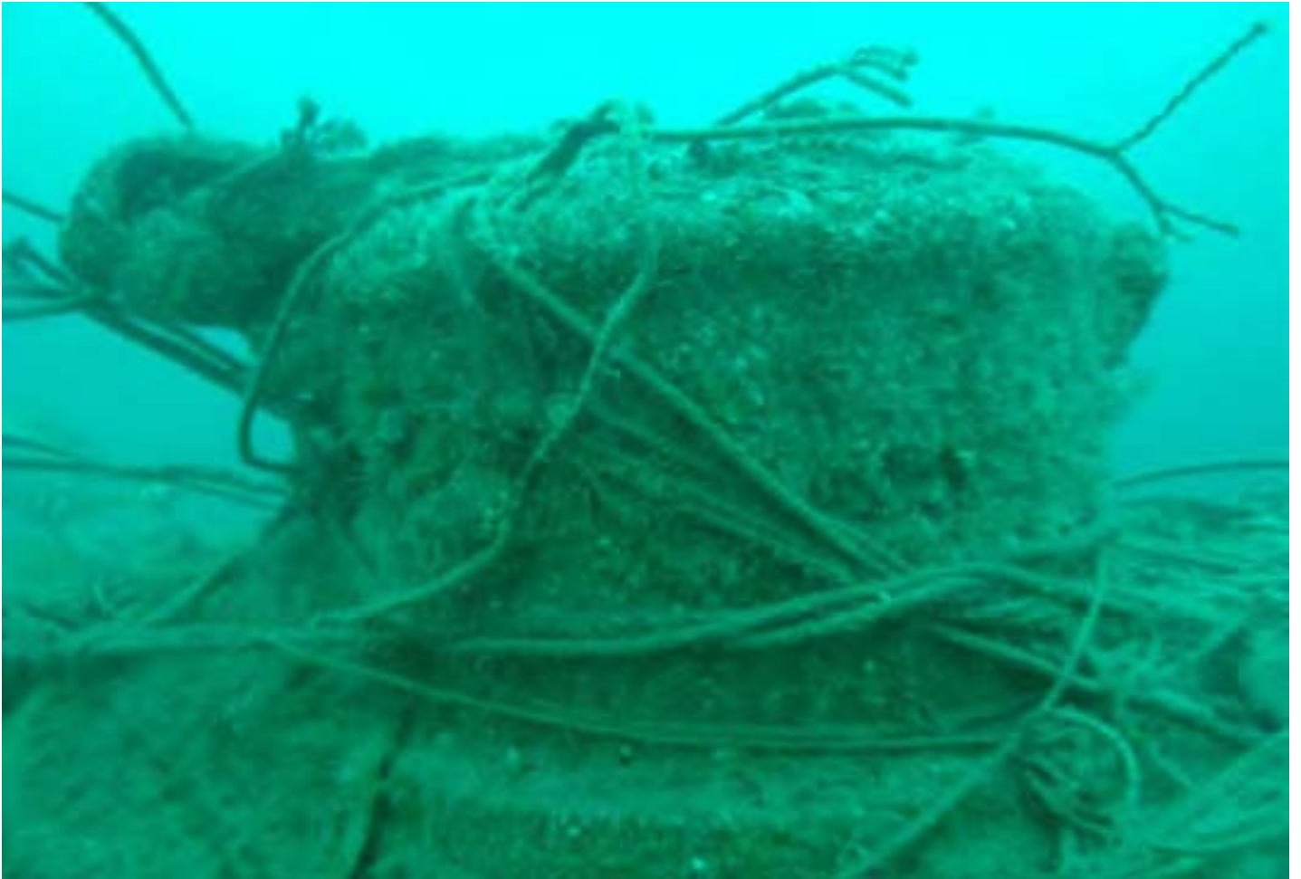
Discarded cable on Holland No. 5 , causing abrasion to the outer casing (Wessex Archaeology).
